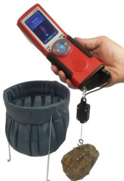
Density Measurement: Sample in Air
