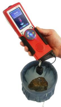
Density Measurement: Sample Submerged in Water
