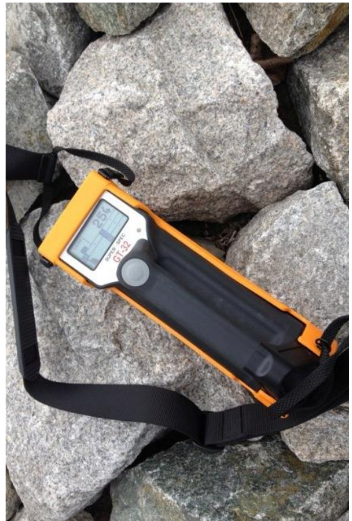
The GT-32 spectrometer comes with a protective boot and a shoulder strap for hands-free surveying
