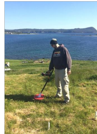
3F-32 Large Diameter Sensor
